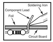
Apply a small amount of solder to the iron tip. This allows the heat to leave the iron and onto the foil. Immediately apply solder to the opposite side of the connection, away from the iron. Allow the heated component and the circuit foil to melt the solder.
