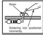
Insufficient solder - let the solder flow over the connection until it is covered.
